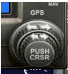
Scroll left until you find the screen that shows the APT EGLL Freqs. Scroll down to find your ILS Freq. (Outside ring scrolls up/down Inside ring scrolls left/right)
