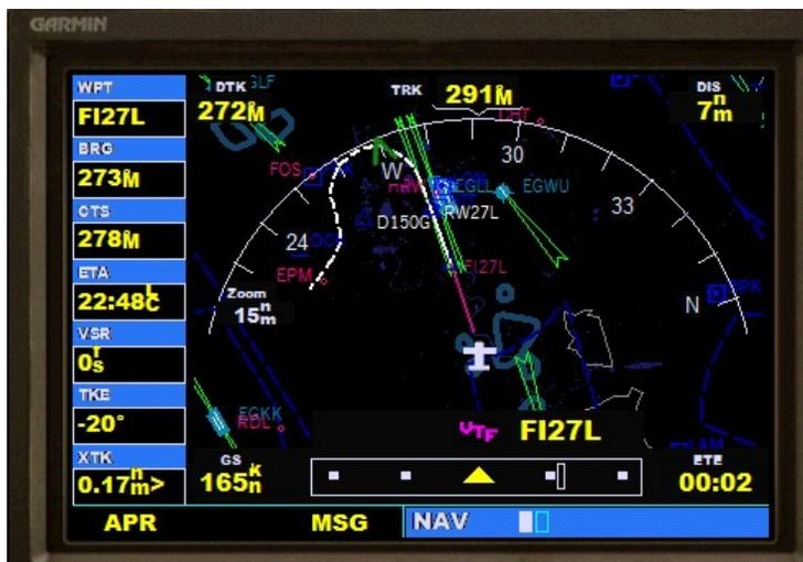
(On the GPS at the bottom right, you'll see XTK 0.17 nm which means I'm .17nm from the Localizer track for Rwy27L. At the bottom middle you'll see the GPS Localizer with the yellow triangle and a bar to the right of the triangle. When the XTK says 1.0nm you need to have the NAV button to ON. You will only see the Localizer on the GPS if you went back into the "Select Approach" screen clicked ENT and chose the ILS - Vectors - Activate This is your "double check" and, you can watch your approach)
